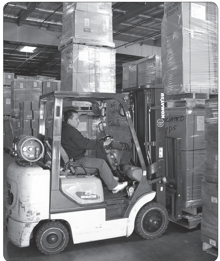
Natural gas is used to power some fork lifts.
